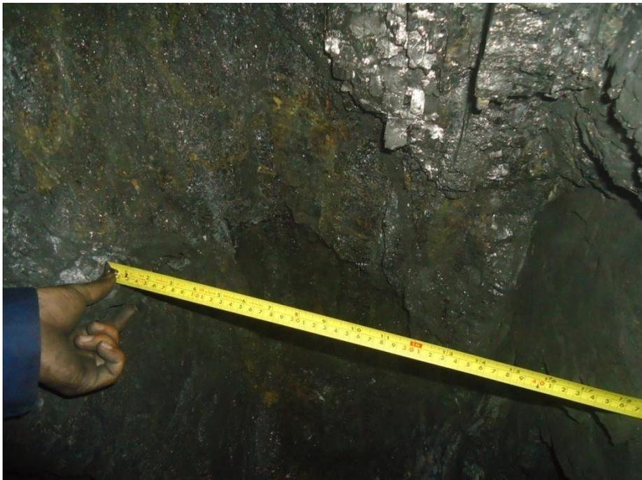
**FOTO 10: Nivel 0 RC4 Coal seam of Luz Angelica width:0.35m. contact:
