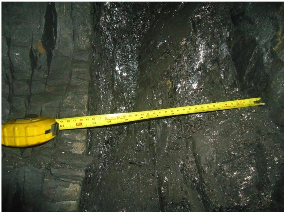
FOTO 12: Nivel 0 RC4, Coal seam of Carito 1 at 770m width: 0.3m. contact: sandstone
