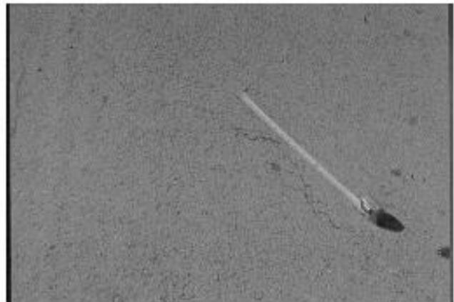
FIG. X1.47 Low-Severity Slippage Cracking
